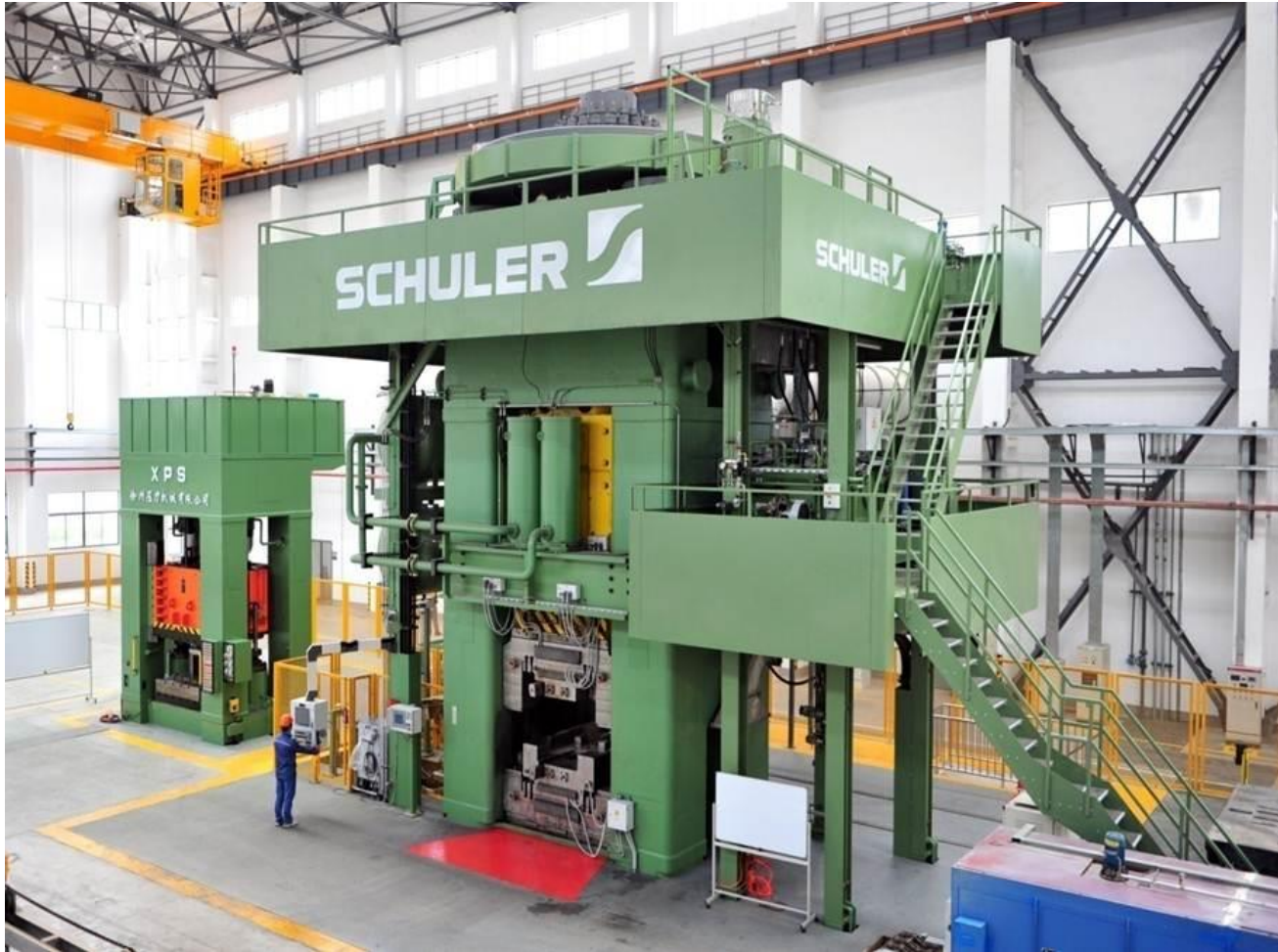
22000T forging machine used by 南车集团, one of the Group's main suppliers
