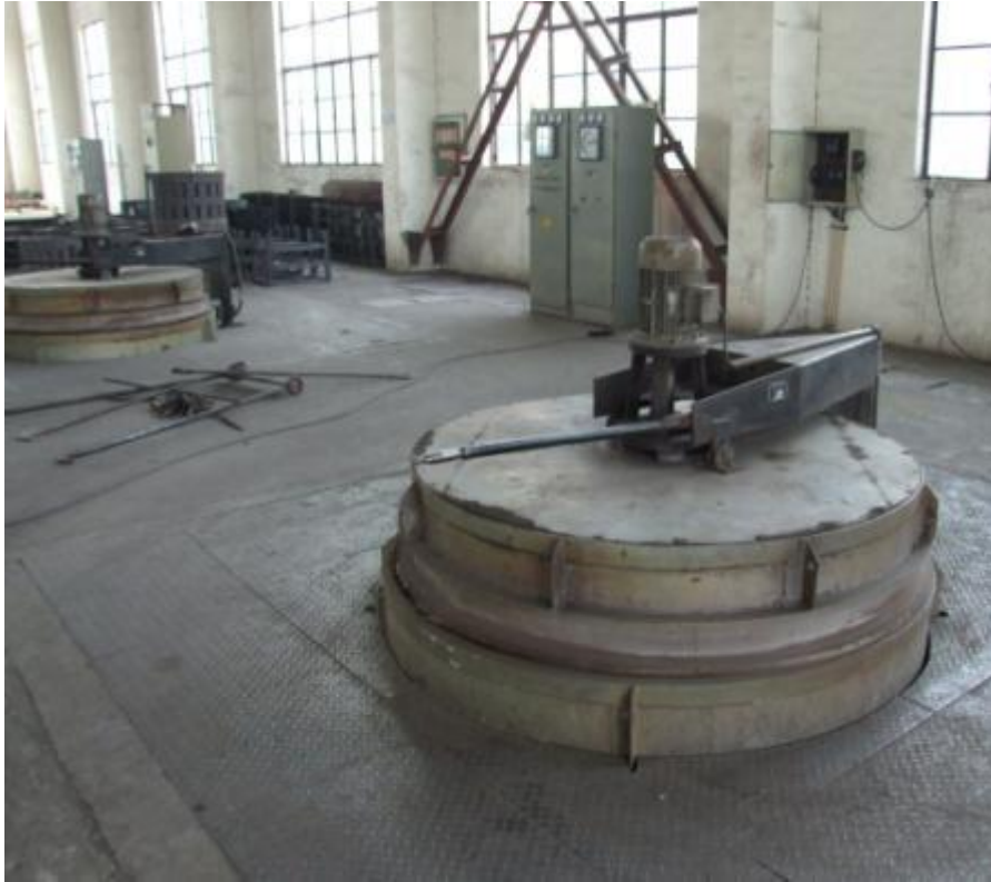
Pit- type Furnace used by 华州锻造 For heat treatment of forged blank. \pm 5^{\circ}\text{C} of variance in temperate control
